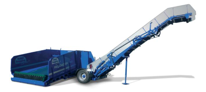
The machine is designed to reload maize silage or other crops from tractor trailer to truck trailers. This machine allows efficient combined transport of the matter from the field to the farm. Combined transport saves costs for fuel, tires, as well as time spent on the road in comparison with tractor transport.
