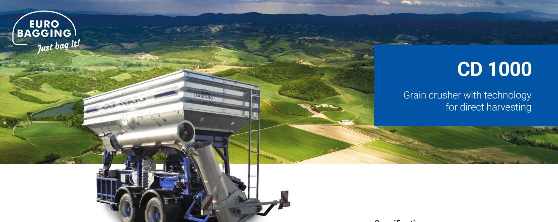
The CD 1000 is designed for crimping wet maize and grain of any kind. Thanks to two rolling units and a massive construction, this crimper has capacity up to 100 t/h.
