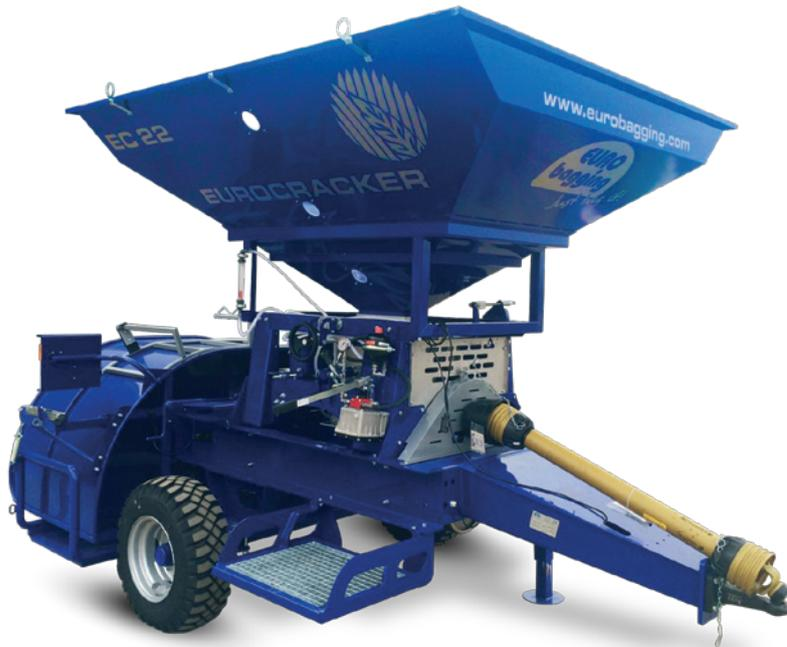
The mobile crimper named the EUROCRACKER is equipped with one crimper unit with V-shaped discs, which do not need as much power in comparison with conventional cylindrical rollers. Thanks to the various circumferential speeds at the disc's junction point, the grain is disrupted better and more evenly. The machine preserves the grain in a bag with a diameter of 1,5 or 2,0 meter.
