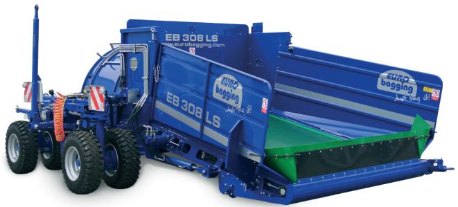
Tractor driven silage bagger designed for grass silage, maize silage, sugarbeet pulps, brewery grain and CCM. Small machine with large usage and high utility.
