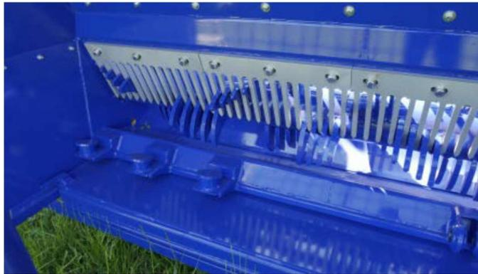
Efficient internal loop braking system, hydraulic bottom cleaning and replaceable counterscreen segments
