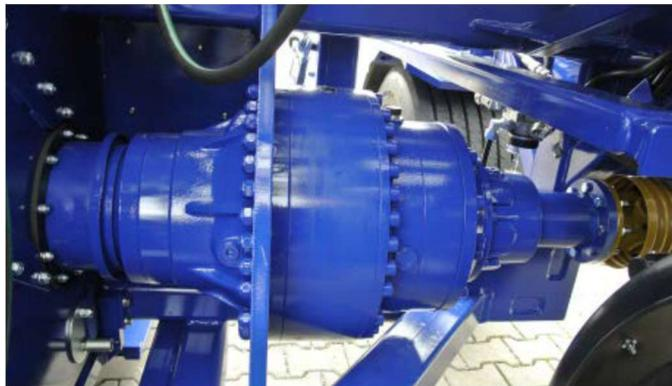
Robust drivetrain with separate gearboxes and replaceable shaft
