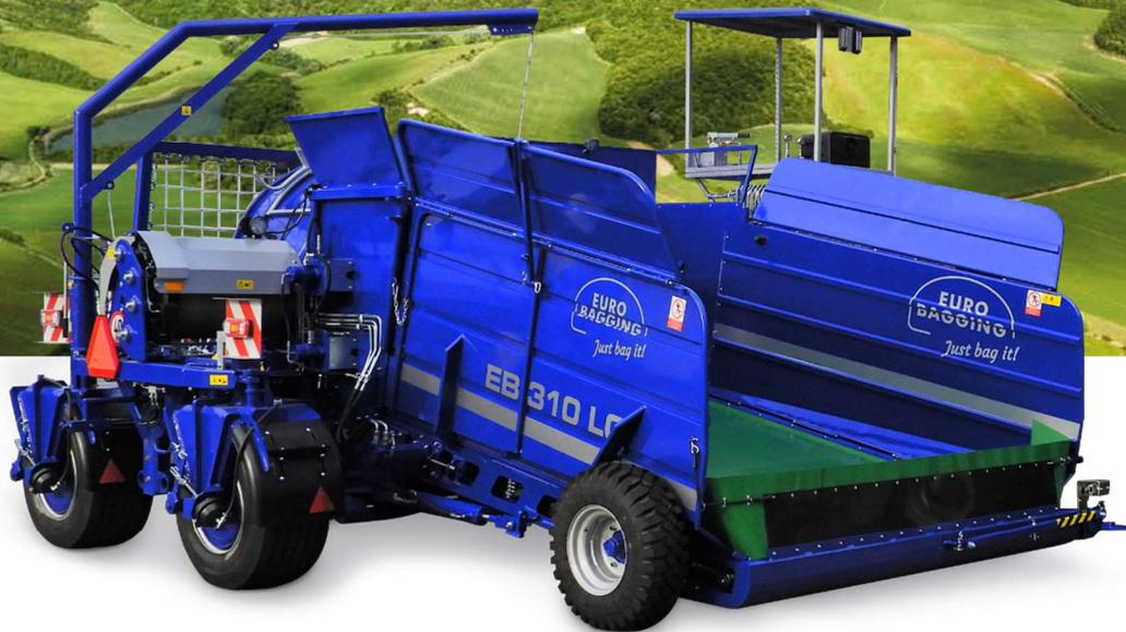
The most popular silage bagging machine of its class for storage of grass haylage, corn silage, sugar beet pulp, CCM or brewing grain. The unique QUICK system allows quick setup of the machine for operation. Convenient hydraulic accessories with proportional control of the main operating functions.
