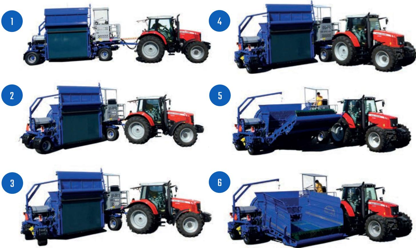
The tractor is attached to the machine at the same point both for both operation and transport. Machine setup after arrival at the work site is much faster and easier compared with other machines.
