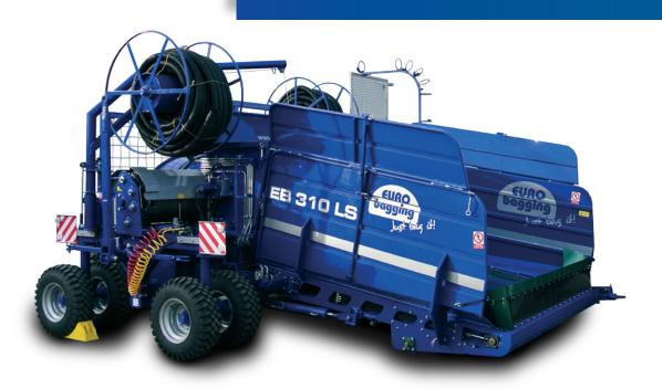
Tractor-driven silage bagger for grass haylage, maize silage, sugar beet pulps, brewer's grain and CCM. Upon request, the machine can be supplied in a composting version.
