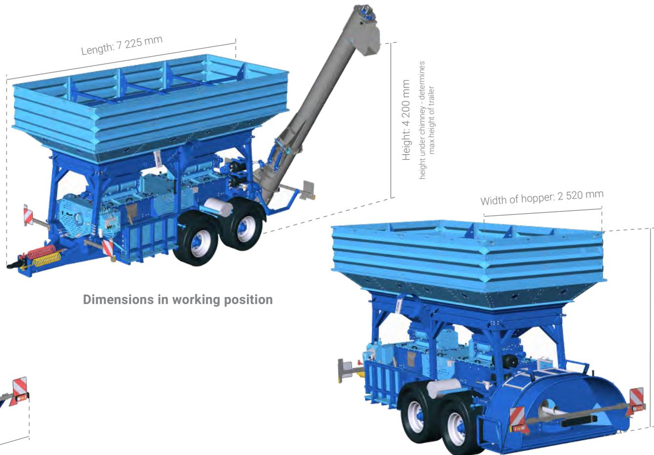
**Dimensions of machine with feed tunnel**
