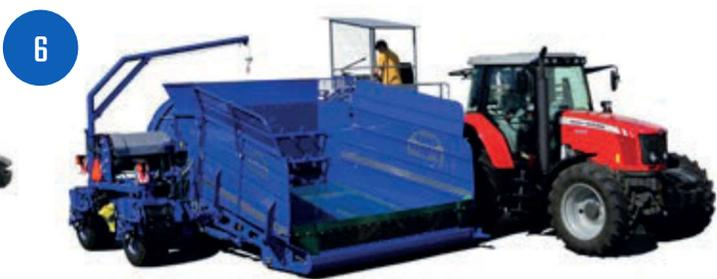
The tractor is attached to the machine at the same point both for both operation and transport. Machine setup after arrival at the work site is much faster and easier compared with other machines.
